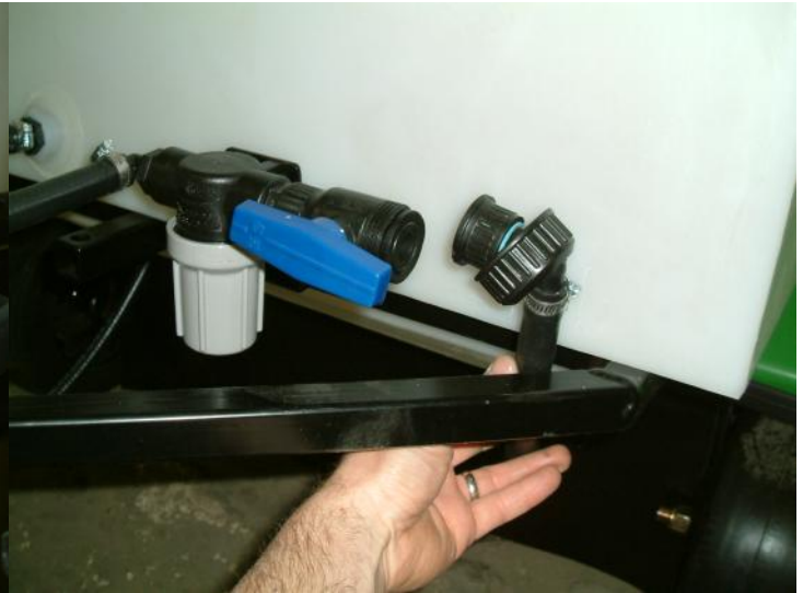
Figure 8: Attaching feed line from tank to valve
