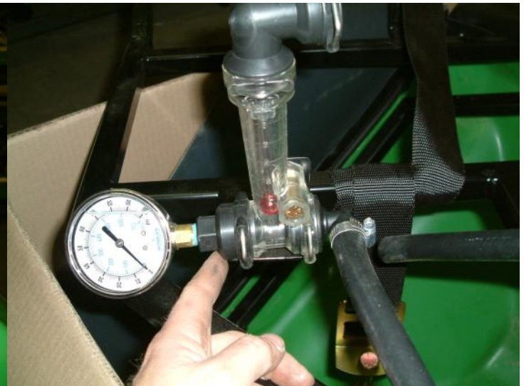
Figure 4: Flow monitor and pressure gauge
