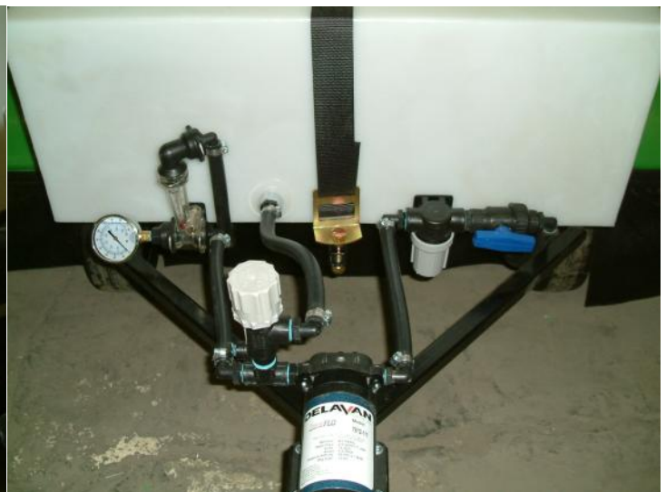
Figure 10: Main plumbing Assembly
