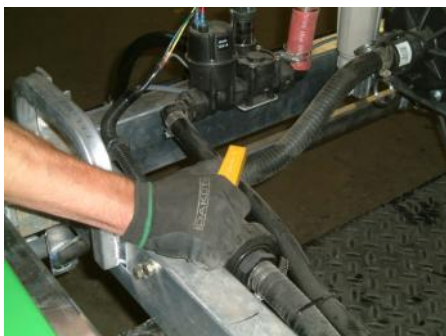
Figure 13. Tank drain ball valve
