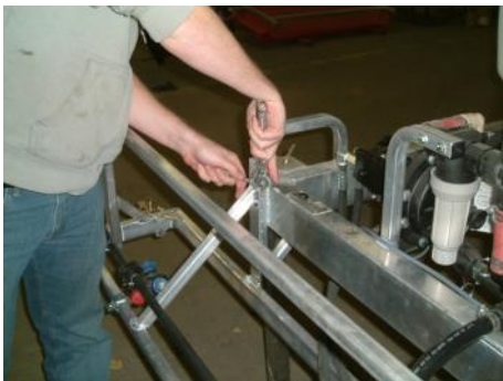
Figure 7. Install center boom
