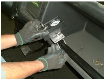
Figure 11. Control box install
