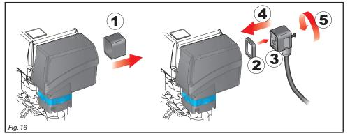
Fix the connectors to the relevant valves according to the initials indicated in your assembly general diagram (7.1 System recommended composition):
