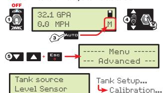
${\bf 3}$   $\,$  From the job screen check that the manual mode is active (the display shows  $\mathbb{M}).$
