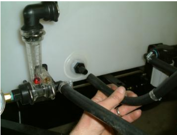
Figure 7: Attaching return line from Pressure Regulator
