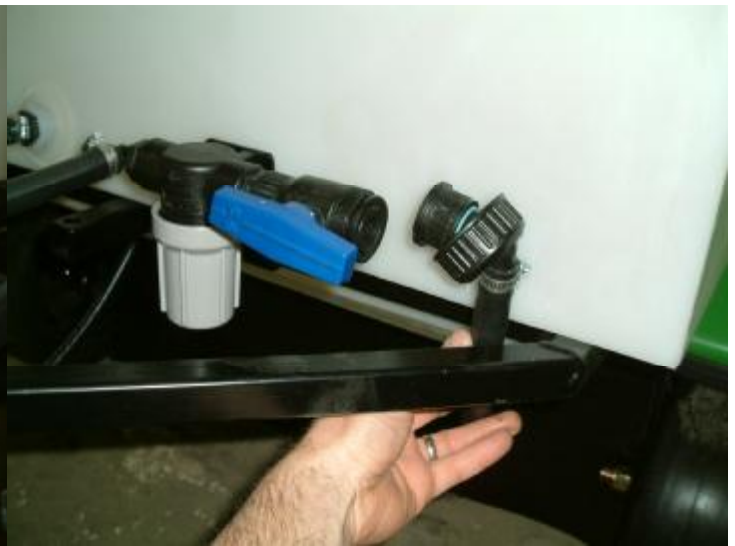
Figure 8: Attaching feed line from tank to valve
