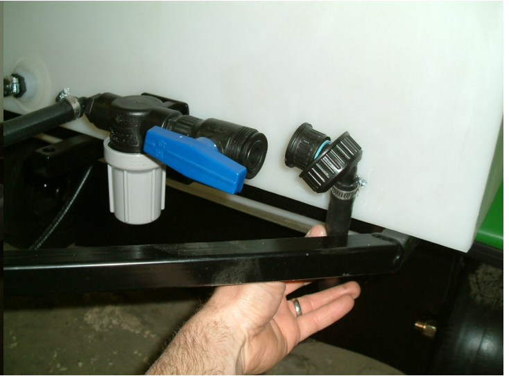
Figure 8: Attaching feed line from tank to valve
