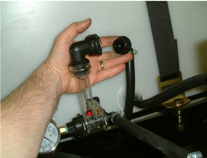
Figure 9: Attaching nozzle feed hose to flow monitor
