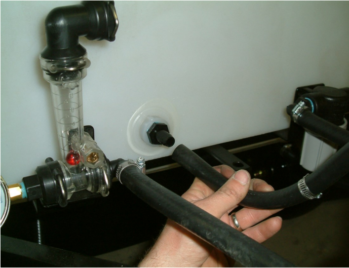
Figure 7: Attaching return line from Pressure Regulator
