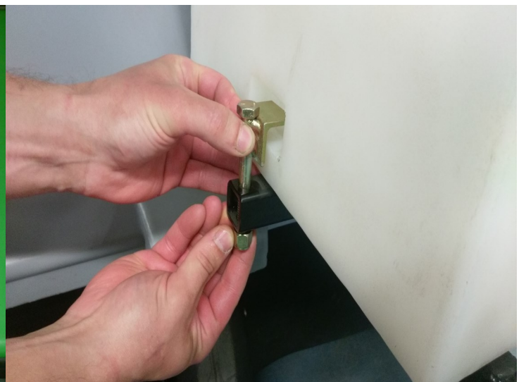
Figure 6: Mount tank and secure with tank locks
