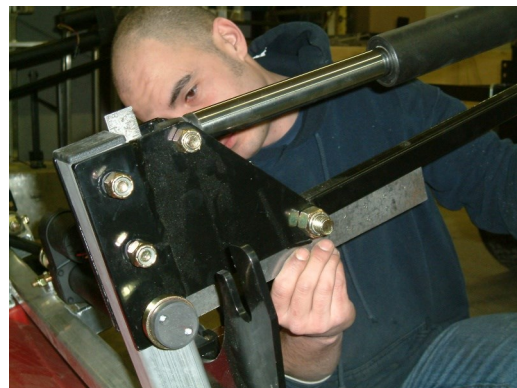
Figure 7: Squaring float arm assembly
