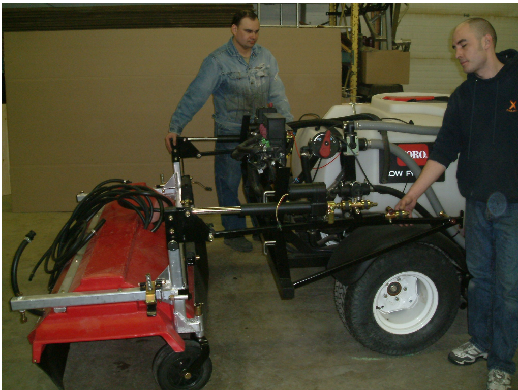
Figure 8: Positioning center section around boom mount assembly
