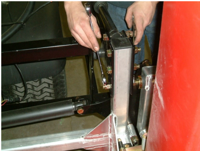
Figure 18: Wing stop adjustment
