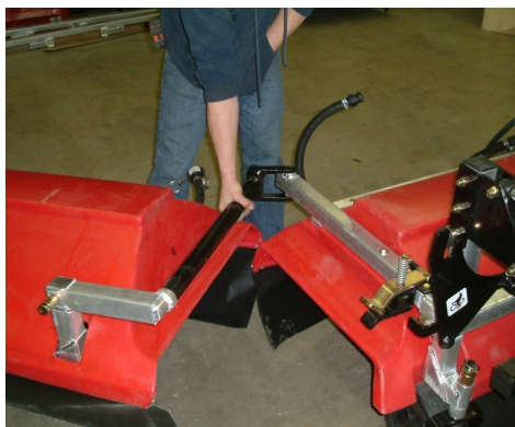
Figure 13: Attaching break away tube to center section
