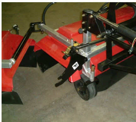
Figure 14: Extend wing actuator
