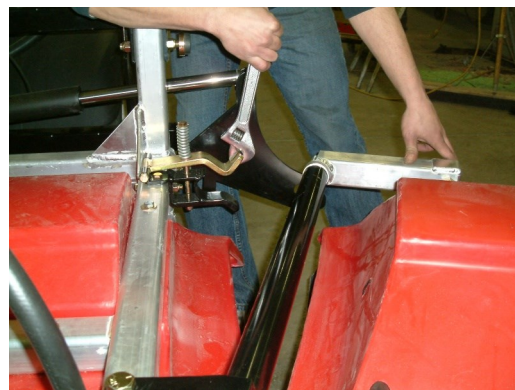
Figure 15: Insert wing into break away catch
