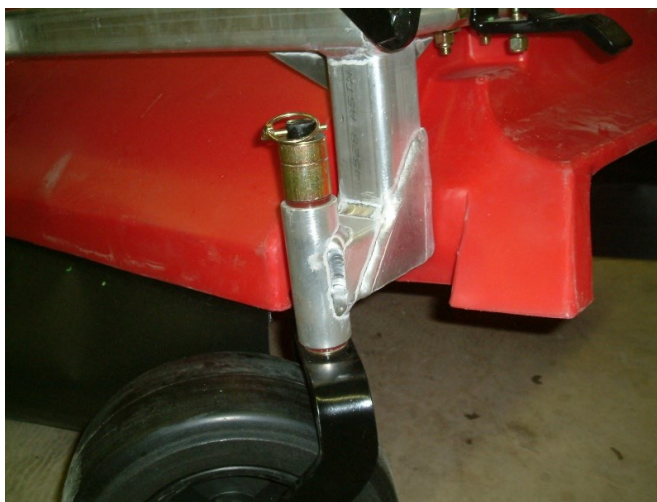
Figure 4: Castor wheel and boom height spacers
