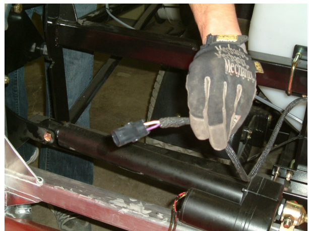
Figure 4: Installed Weather-Pak end
