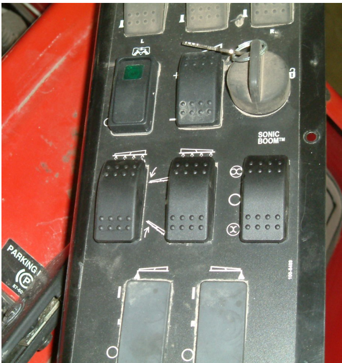
Figure 21: Rocker Switches in Console Panel
