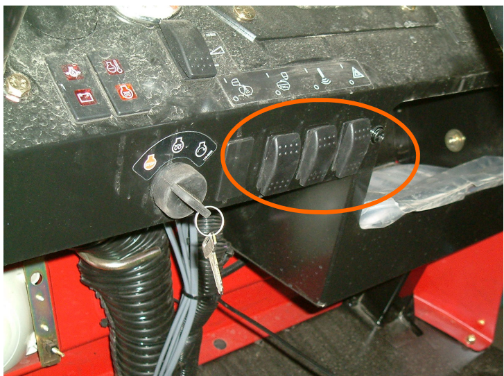
Figure 23: Dash of 5800 with inserted switches
