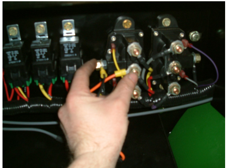
Figure 22: Power wire attachment locations
