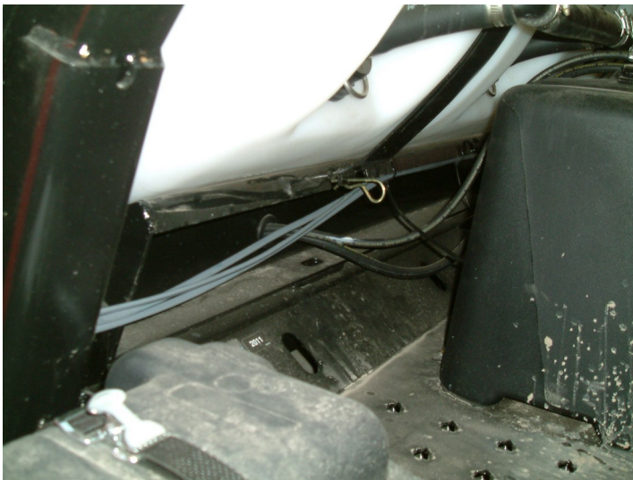
Figure 26: Wire placement along tank
