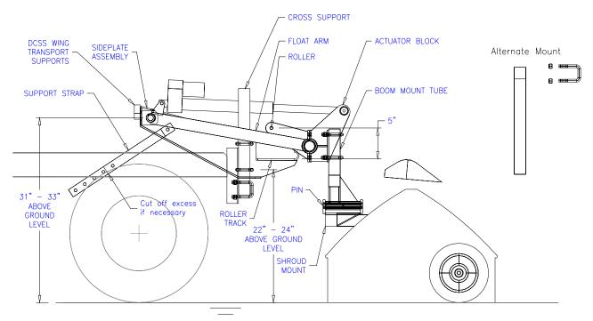
If the mounting area on the prime mover is too high, the cross support can be inverted so the boom hangs below the mounting point. Adjust the U-bolts on the cross bar and on the boom mount so that the boom is level when standing on level ground and there is approximately 4 ½" between the roller and the track it follows on the sideplate.
