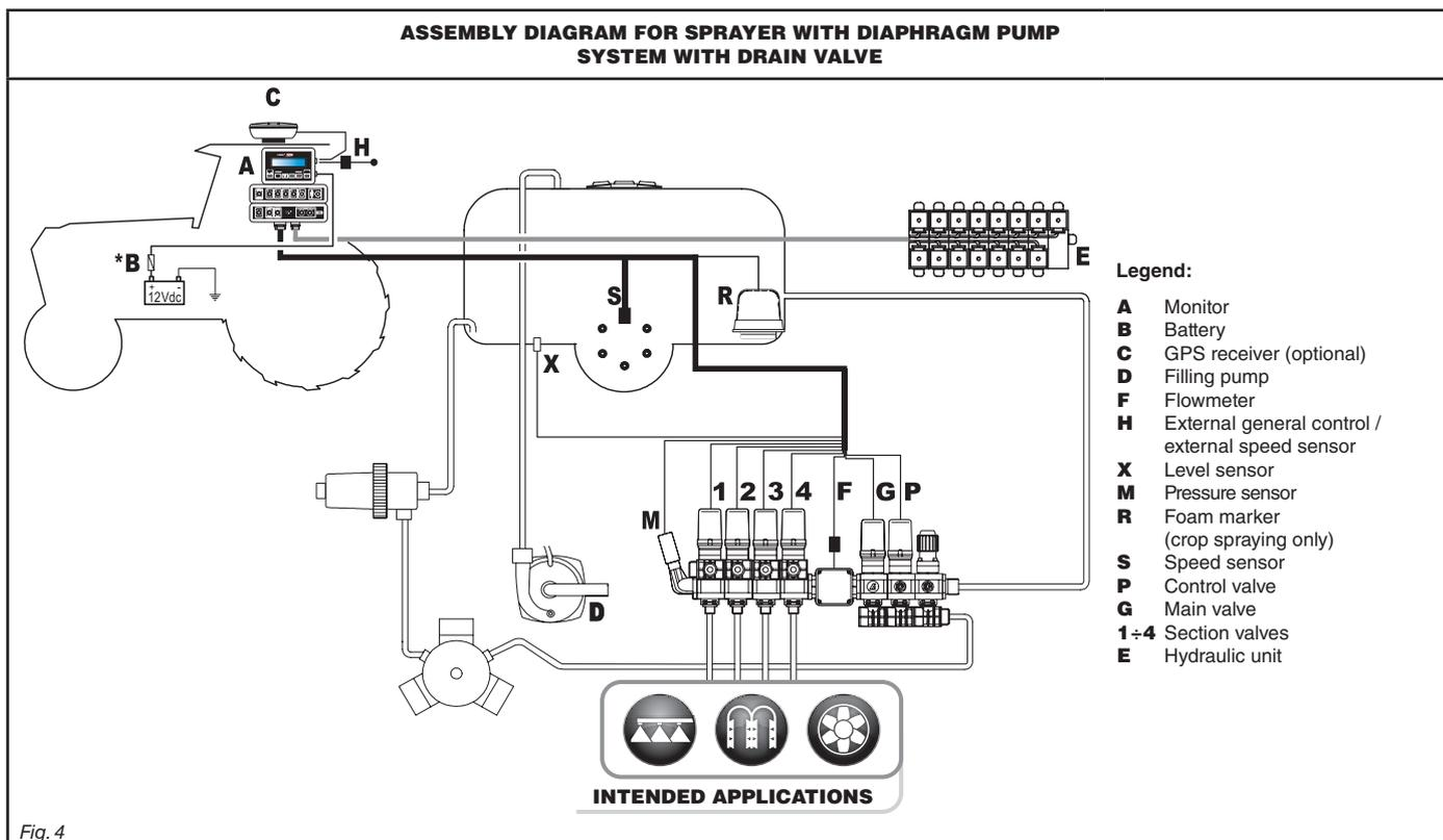
The computer must be directly connected to the farming machine battery.
