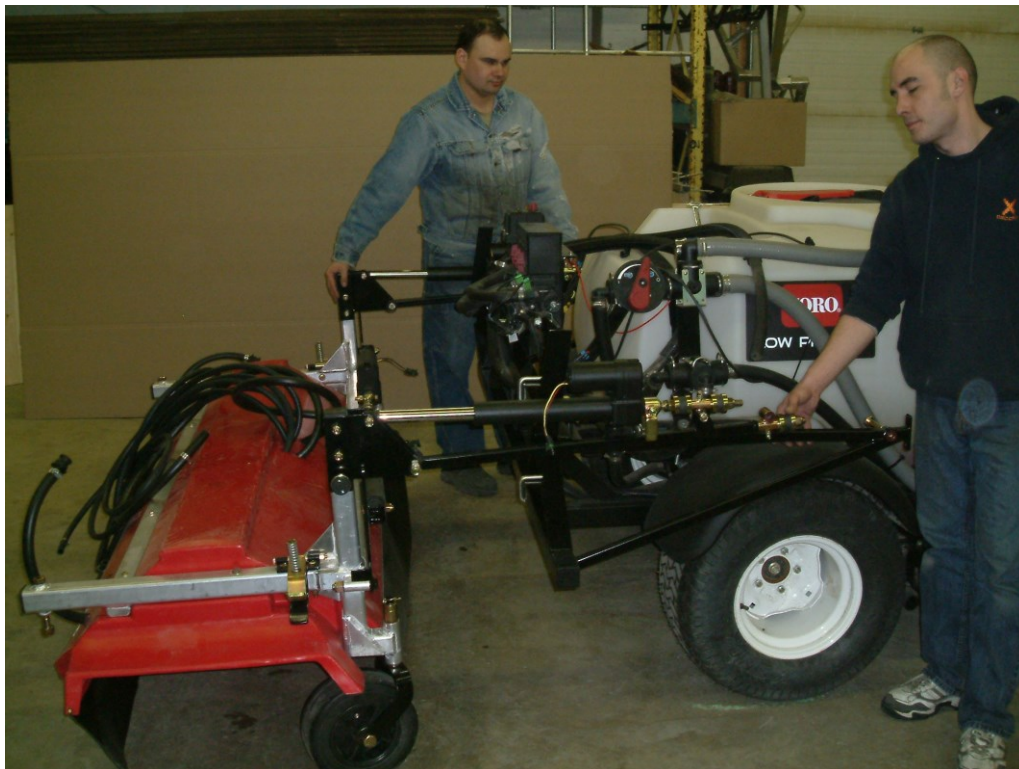
Figure 8: Positioning center section around boom mount assembly
