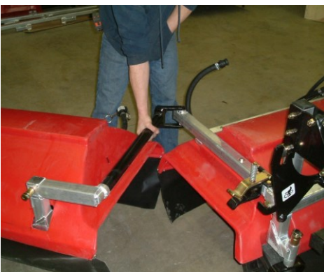
Figure 13: Attaching break away tube to center section
