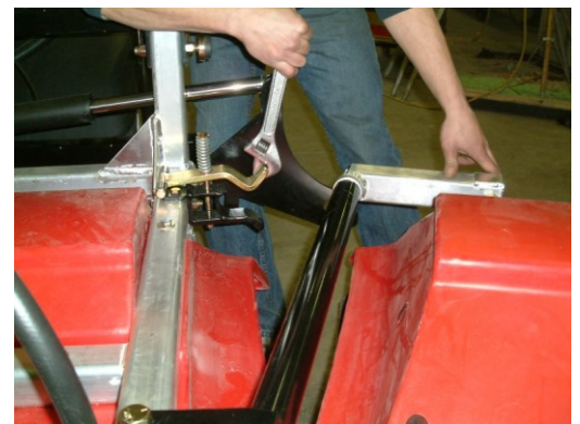
Figure 15: Insert wing into break away catch
