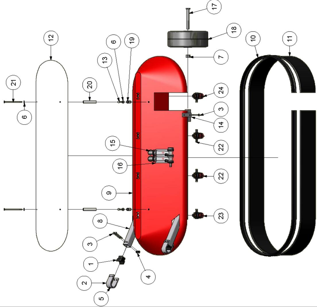
NOTE: STANDOFF BOLTS HELD ON INSIDE WITH WASHER AND LOCKNUT (#00968 & #01157)
