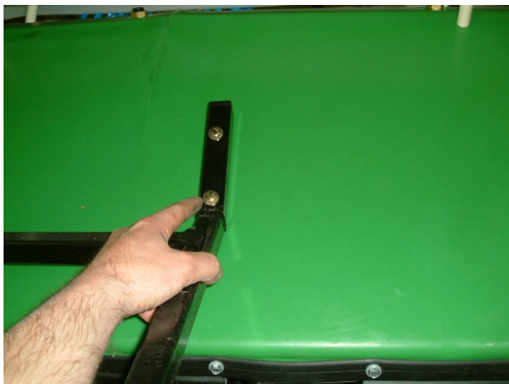
Figure 5: Mounting hitch on boom
