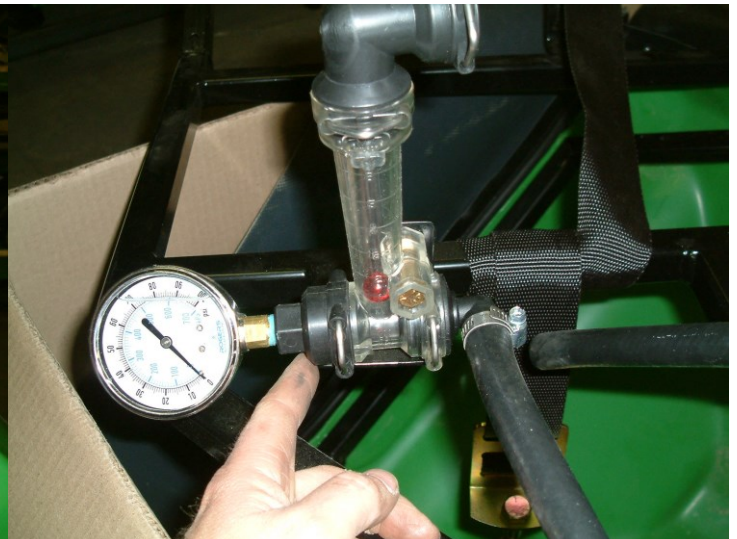
Figure 4: Flow monitor and pressure gauge
