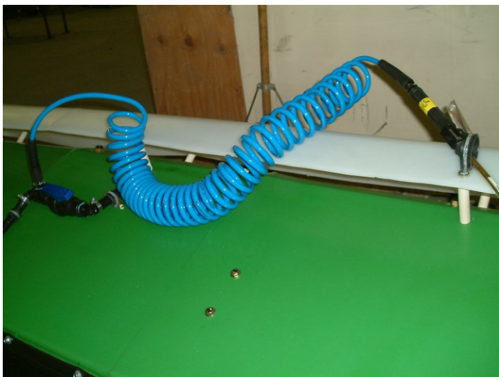
Figure 13: Spray wand holding clamps
