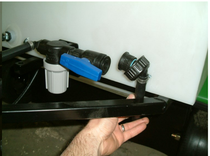
Figure 8: Attaching feed line from tank to valve
