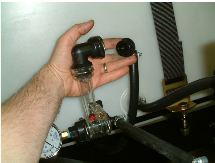
Figure 9: Attaching nozzle feed hose to flow monitor
