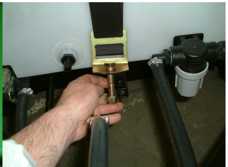
Figure 6: Mount tank and secure with strap
