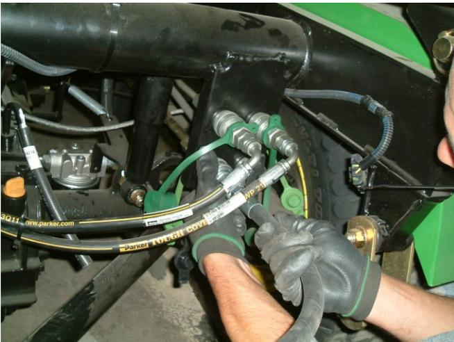
Plug in the hydraulic lines to the female outlets underneath your work vehicle
