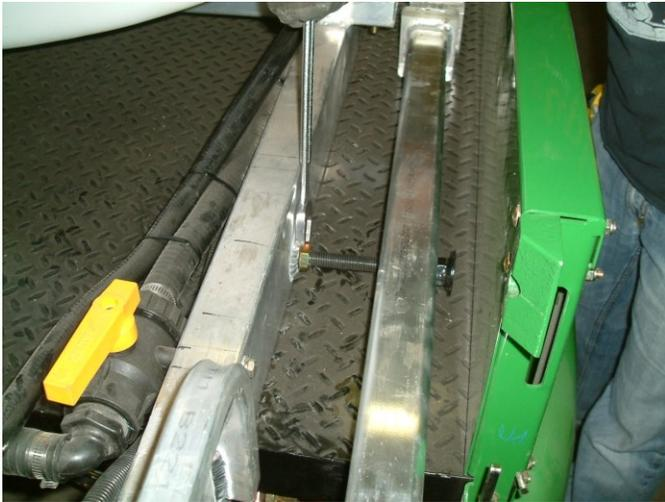
Center sprayer in box and thread out tank locks so that skid is firmly in box. Use jam nut to hold threaded tank lock in place. Skid frame should be tight against the front of the box.
