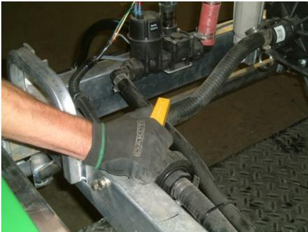
Figure 8. Tank drain ball valve
