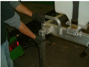
Stand unit up using legs and pins as seen in Figure 1.
