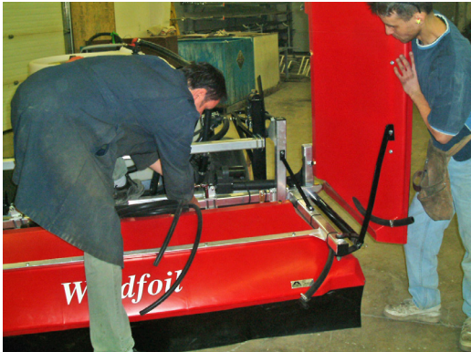
Setting Actuator Mount Bracket
