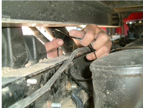
Attach Wires to Frame, Avoid Exhaust
