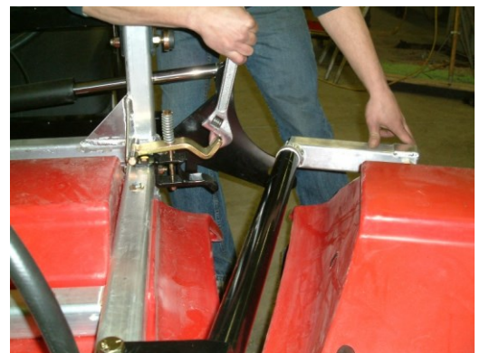
Figure 15: Insert wing into break away catch
