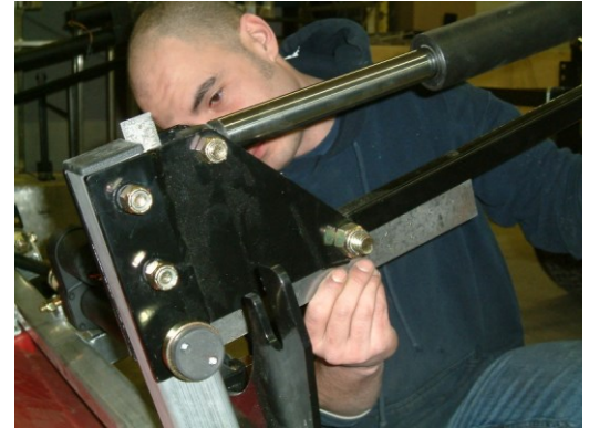
Figure 7: Squaring float arm assembly
