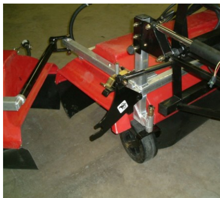
Figure 14: Extend wing actuator
