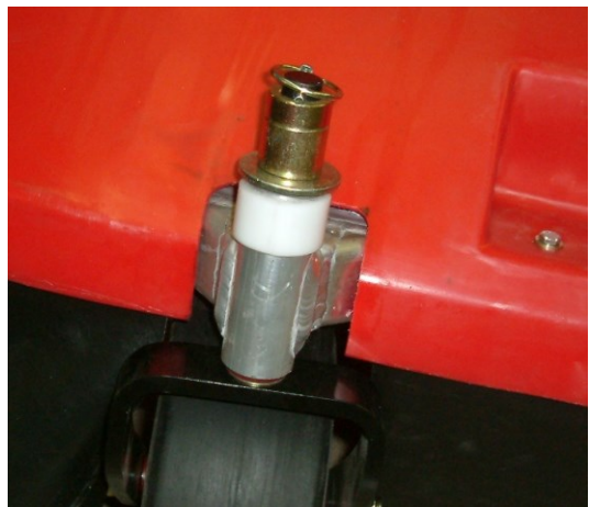
Figure 12: Wing Castor Wheel
