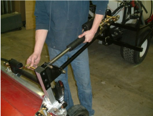
Figure 5: Float arm assembly
