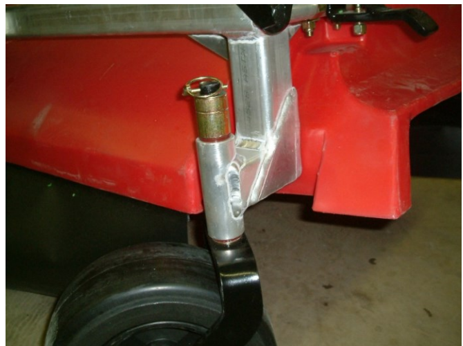
Figure 4: Castor wheel and boom height spacers
