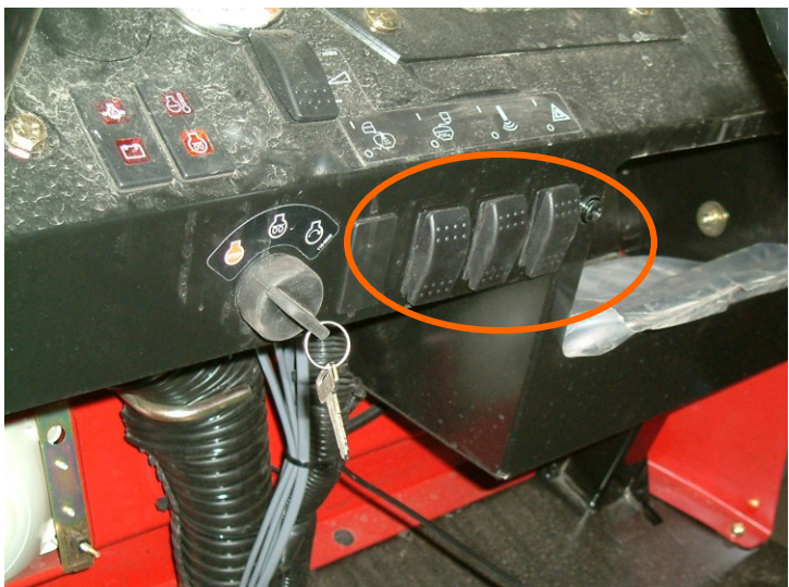
Figure 23: Dash of 5800 with inserted switches
