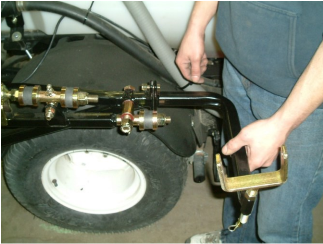
Figure 16: Wing support arm
