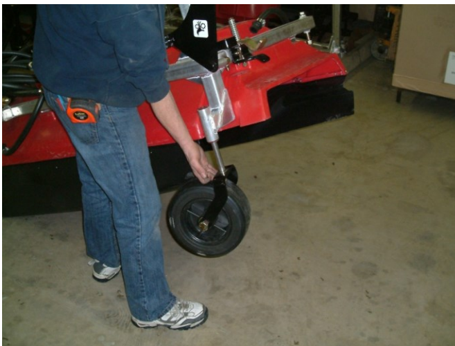
Figure 3: Inserting castor wheel
