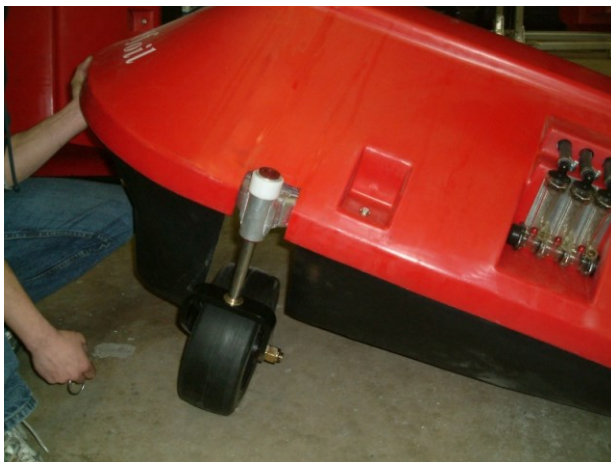
Figure 11: Wing castor wheel
