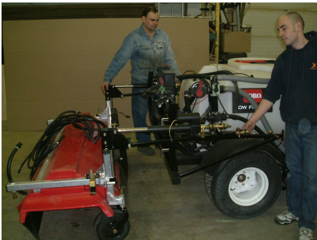
Figure 8: Positioning center section around boom mount assembly
