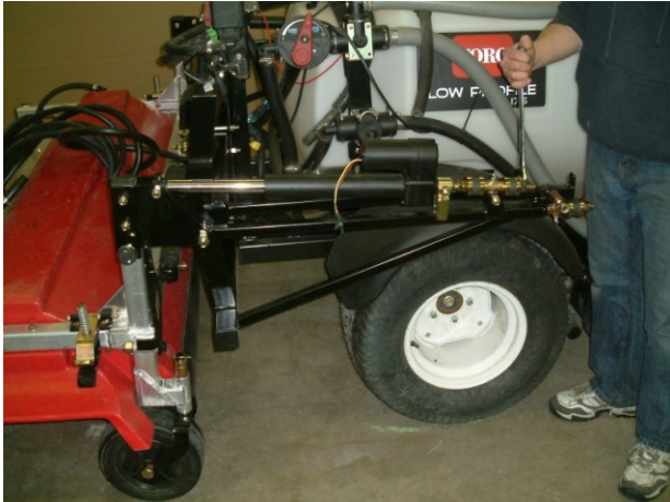
Figure 9: Center Section adjustment
