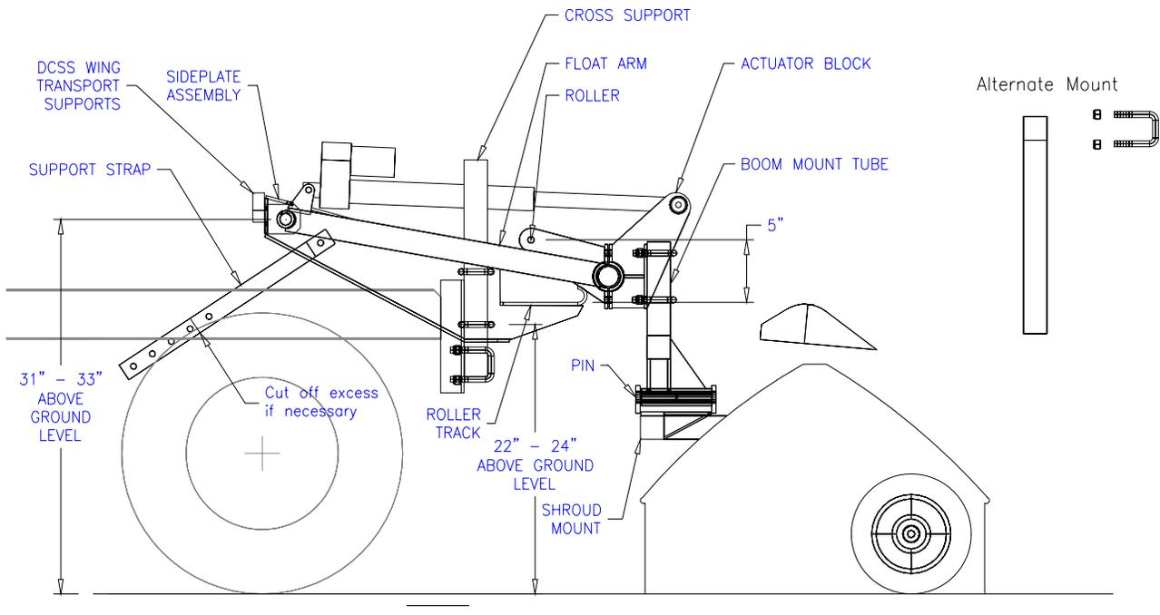
If the mounting area on the prime mover is too high, the cross support can be inverted so the boom hangs below the mounting point. Adjust the U-bolts on the cross bar and on the boom mount so that the boom is level when standing on level ground and there is approximately  $4\frac{1}{2}$ " between the roller and the track it follows on the sideplate.
