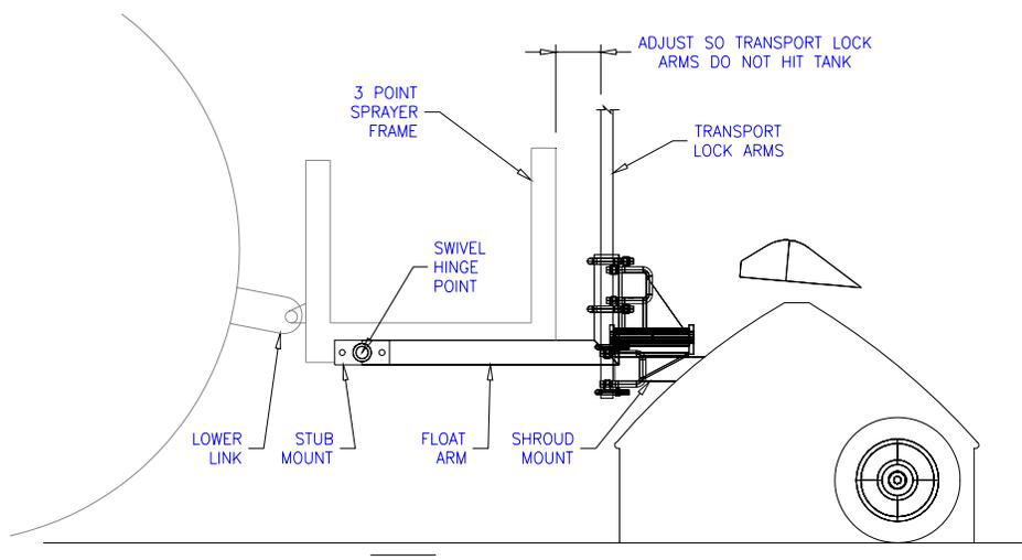
Adjust the float arms on the pivot frame so the boom is level when the 3 point hitch tractor sprayer bottom is 12" – 18" off the ground.
