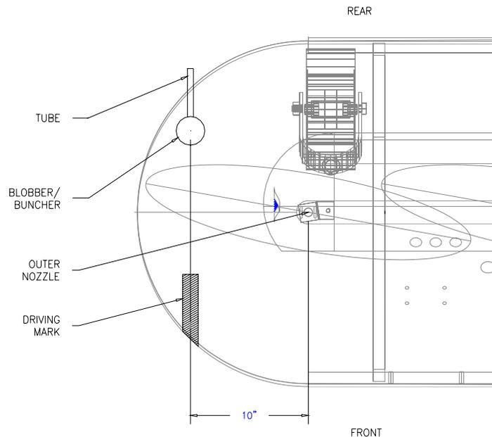
Under certain conditions large foam blobs will suffocate the grass underneath them. This can be minimized by smearing the foam and by using the smallest blob possible. Some operators replace the large blobber supplied with a 1/2" hose running down the back edge of the curtain.
